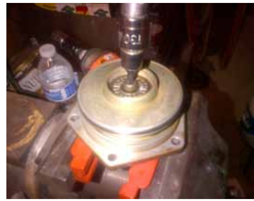
Figure 8 Removing center bolt
