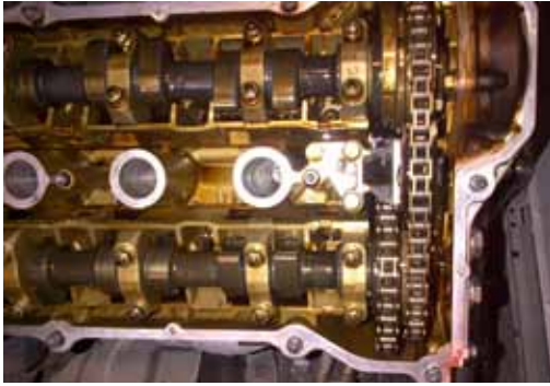
Figure 4 Cam lobe position when at OT
