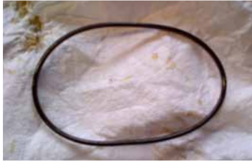
Figure 6 Distorted shape of original o-ring
