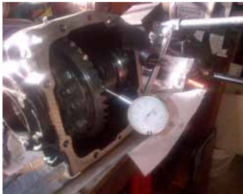
Figure 4 Backlash check with dial indicator on magnetic base
