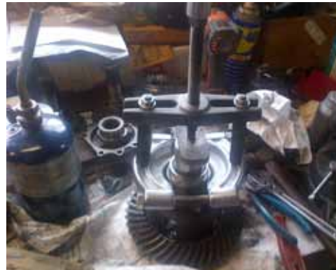
Figure 2 Bearing puller to remove race
