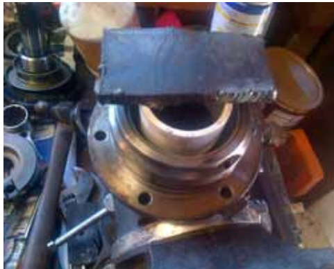
Figure 1 Pushing seal out
