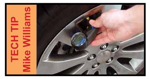
$\overline{\mathbf{I}}$  ire pressure is a measure of the amount of air in a vehicle's tires, in pounds per square inch. The required service involves checking the tires' pressure with a pressure gauge, at least monthly, if not more frequently.
