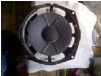
FIGURE 10 OLD FOAM REMOVED
