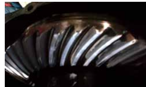
Figure 11 Contact pattern after a few rotation
