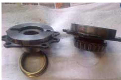
Figure 7 Left is replacement modified flange, Right is original height
