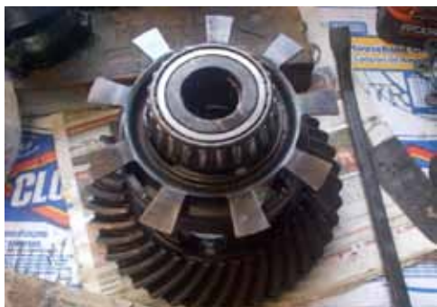
Figure 13 LSD differential removed with right side up
