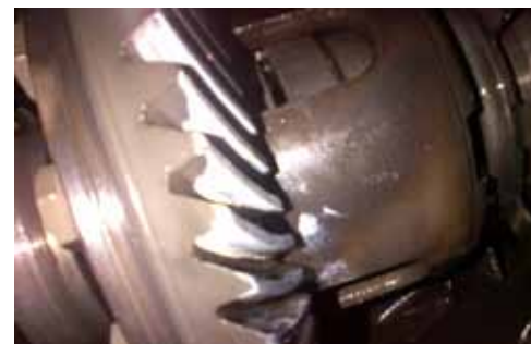
Figure 10 Gear marking paint to check gear pattern
