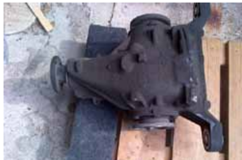
Figure 1 Final Drive removed from car
