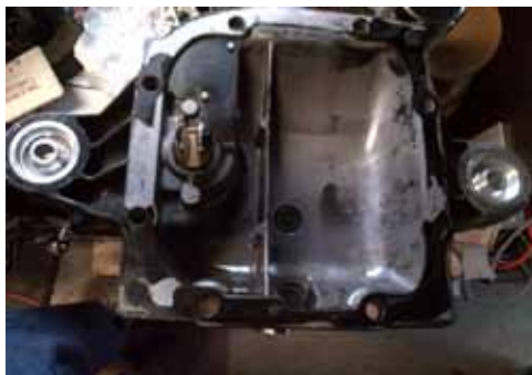
Figure 5 Rear cover and crumbled gasket
