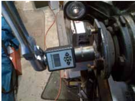
Figure 4 Torque check before disassembly
