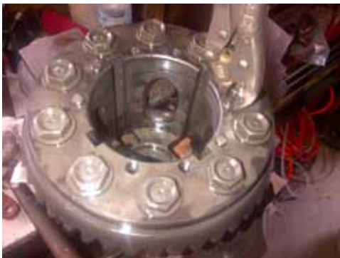
Figure 15 Removing broken flange bolts
