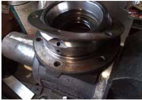
Figure 12 Output flange, O-ring, shim and bearing inner race
