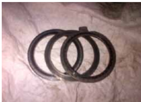
Figure 16 washer, Bellville spring, and keyed washer
