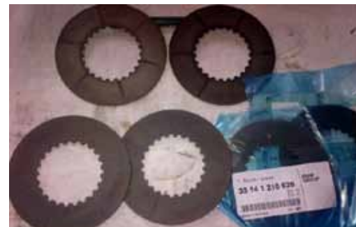
Figure 18 Friction plates, used plates at top
