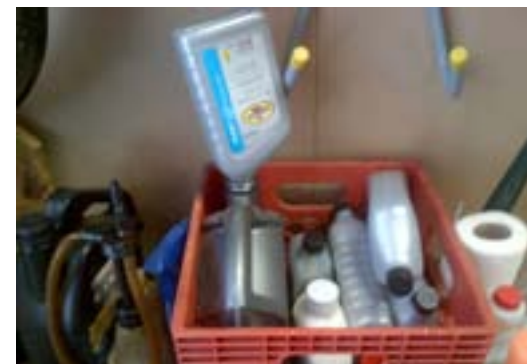
Figure 4 Oil draining, reduces waste in landfill
