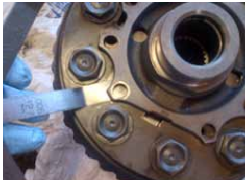
Figure 6 Check of shaft Bellville washer spacing w/.005 feeler gauge
