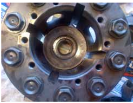
Figure 4 Differential body with shaft washers, large Bellville washer installed
