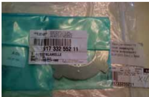
Figure 1 Porsche Outer Disc or dog ear plate
