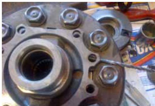
Figure 7 Drill bit check of flange to body gap
