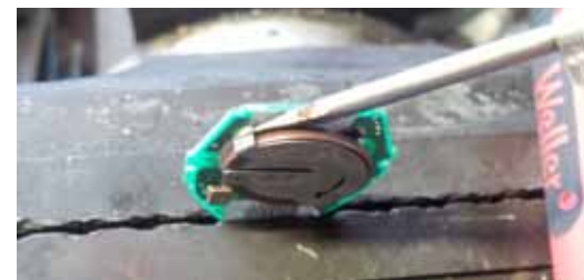
Figure 6 De-solder old battery
