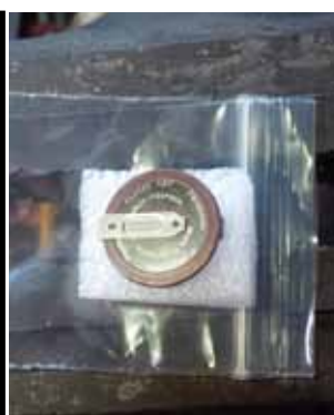
Figure 2 replacement battery, with wrong pin out
