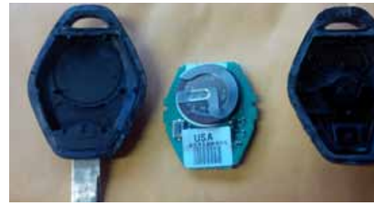
Figure 5 Circuit board out, note 90 deg pin out
