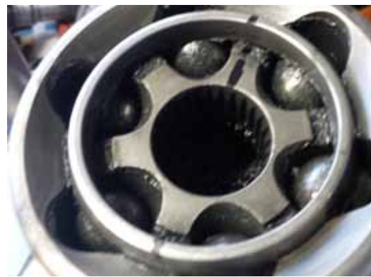
Figure 10 Inside CV joint with orientation marks
