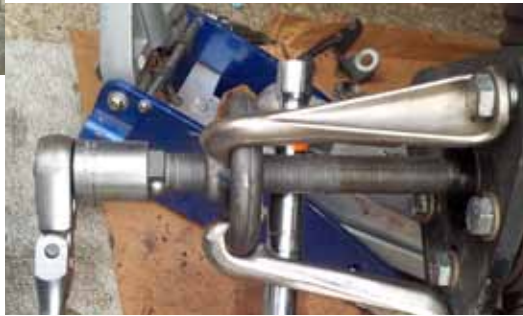
Figure 8 Axle remover, bolts to hub and pushes spline out
