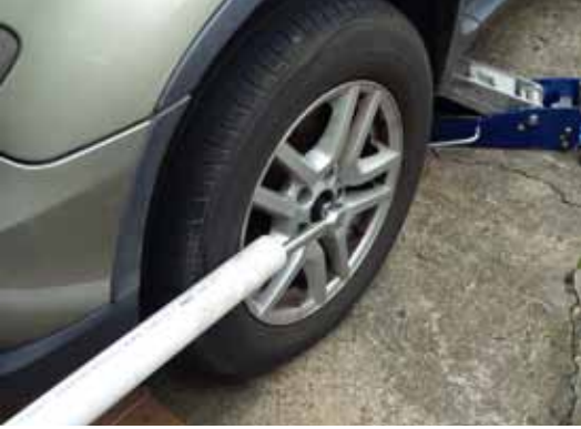
Figure 5 Set up to break axle nut, ¾ breaker bar and 2" PVC pipe
