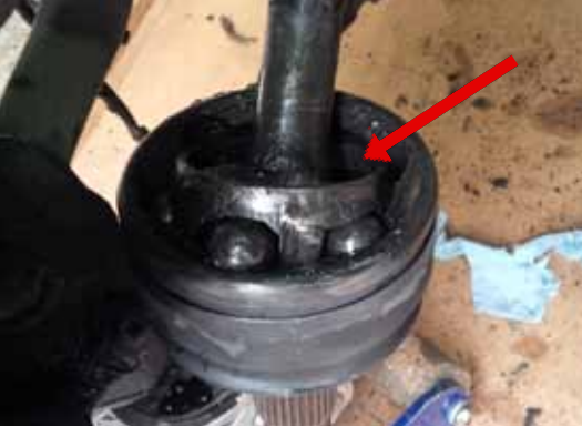
Figure 9 CV ready to tap apart, tap at end of arrow on spline ring
