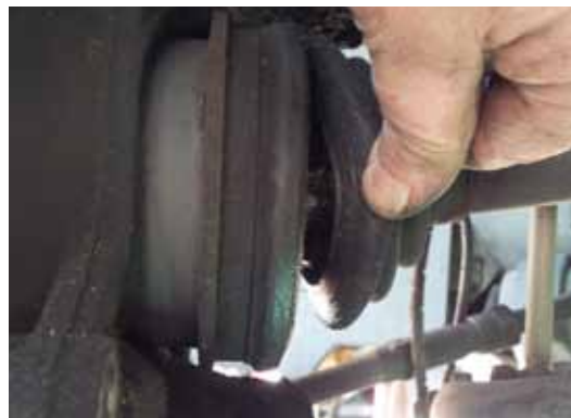
note grease still in the joint
