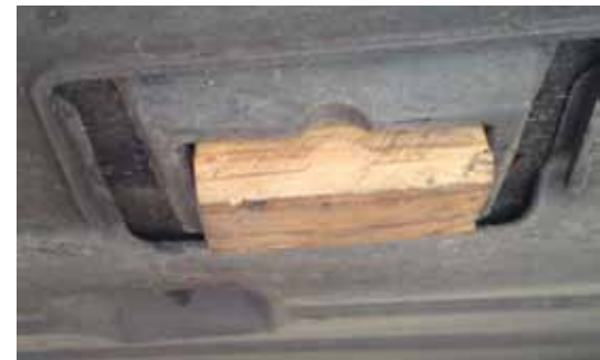
damage to the plastic piece on the jack points
