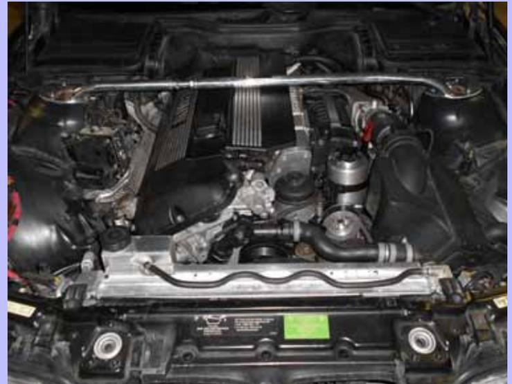
engine without requiring any change to the internal structure. Because it is a twin screw blower it starts providing boost as soon as the turbines are spinning and reaches full boost potential (8.5psi) at 2200 rpm. I did the install myself and it took me about a week.
