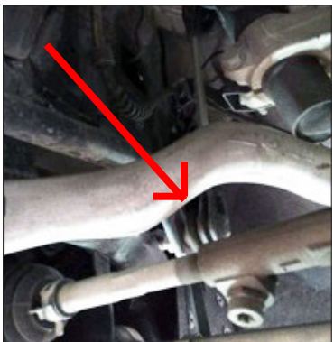
FIGURE 2: E30 standard link to control arm, reduces bar effectiveness to reduced movement of bar end and rubber at clevis bolt connection
