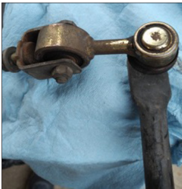
FIGURE 2: E30 standard link to control arm, reduces bar effectiveness to reduced movement of bar end and rubber at clevis bolt connection
